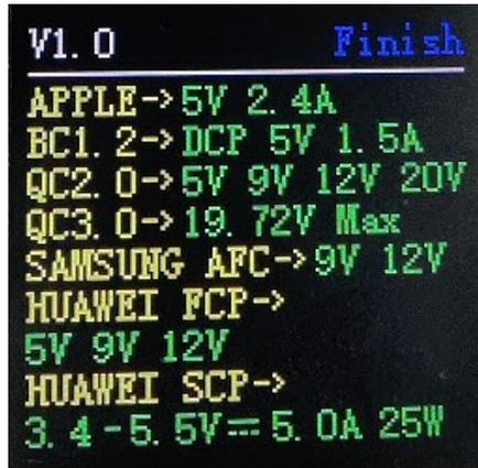
In this mode, the meter tries to trigger various protocols in turn, and displays the test results on the screen. Red means not supported, and green means supported. During the test, it is forbidden to connect to any equipment at the back end.
