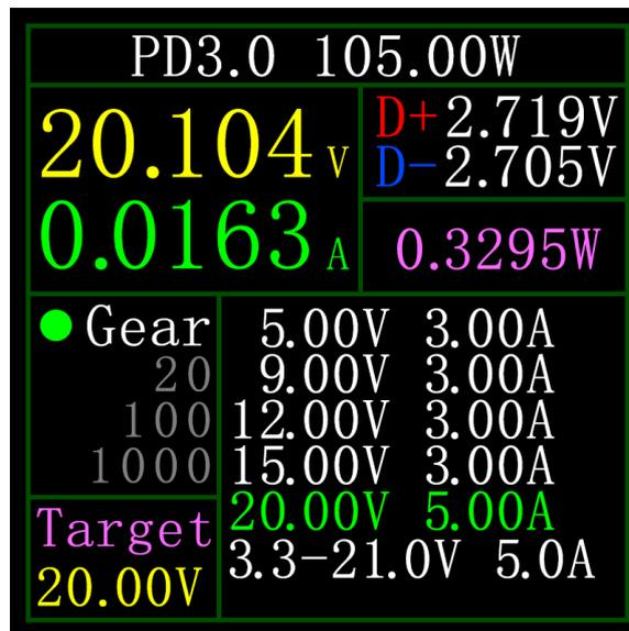
Take the picture as an example. The picture shows a charger sending a message with a total of 6 gears, among which gears 1, 2, 3, 4, and 5 are fixed voltage gears, and gear 6 is adjustable voltage gear (PPS).
