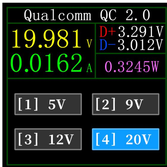
In QC2.0 trigger mode, use the left and right keys to select the trigger voltage, and long press the OK key to return.
