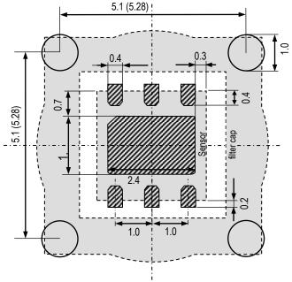
**Figure 3**: PCB layout example of SHT2x and filter cap SF2; all DFN sensors of smaller size to be placed according to the example in the center of the SF2 outline. Dimensions are given in mm (1mm = 0.039 inch). The distance of the openings is 5.1mm  $\pm 0.05$ mm if the sensor should clip on the PCB and 5.28mm if the pins are used for adjustment only. By varying the openings distance about  $\pm 0.05$ mm the clipping force may be adjusted.
