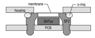
**Figure 2:** Side view of SF2 filter cap mounted between PCB and housing wall. The volume below the membrane is kept minimal and the membrane is separated from the surrounding volume enclosed by housing.
