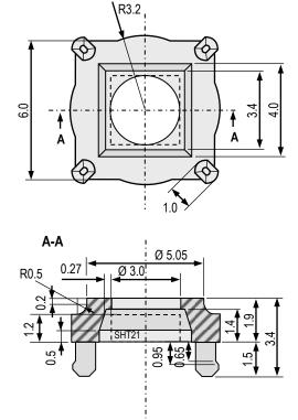
**Figure 1:** Drawing of the filter cap SF2 (body only). Dimensions are given in mm (1mm = 0.039inch), tolerances are  $\pm 0.1$ mm. Add 0.15 to total height due to the filter membrane. The cavity inside the cap fits to SHT2x/3x/4x, SHTC1 and SHTC3 sensors. Additional space for solder joints are left open around the sensor.
