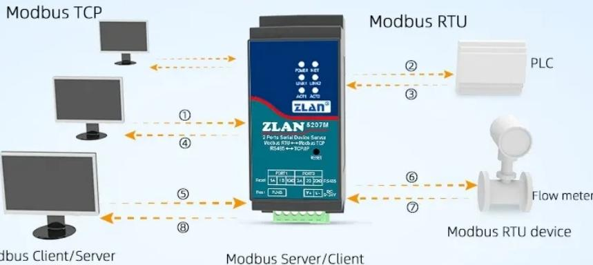
It is used as the Modbus TCP slave station when the working mode is TCP Server
