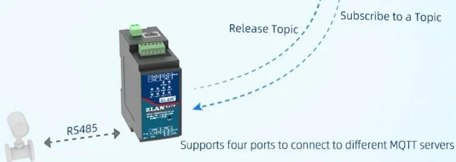
Transparent transmission mode : The subscription information and serial port data are transparently-transmitted to each other.
