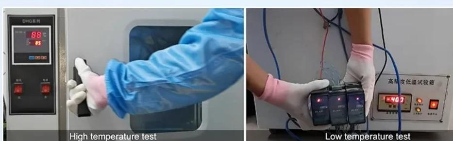
It works normally at high temperature of 85°C Low temperature -40°C stable operation
