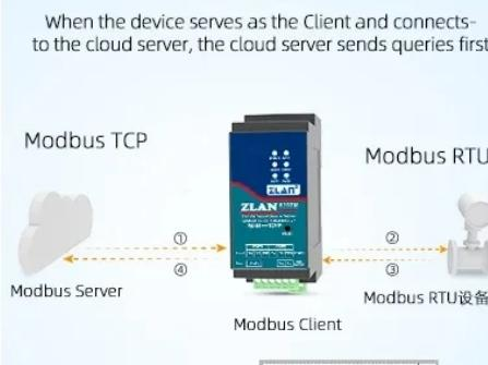
When the device serves as the Client and connects to the cloud server, the cloud server sends queries first
