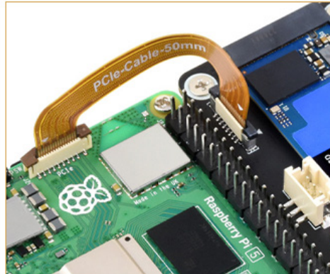
Power supply via PCIe cable
