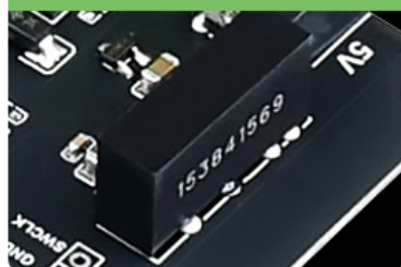
Power Supply Isolation
