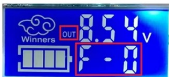
F-0 indicates the display output voltage
