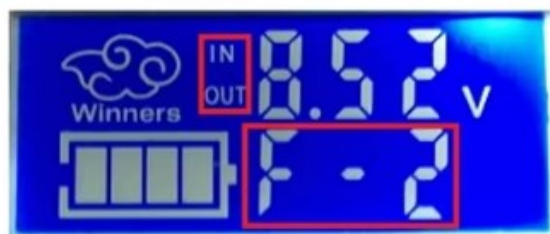
F-2 indicates switching display input and output voltage
