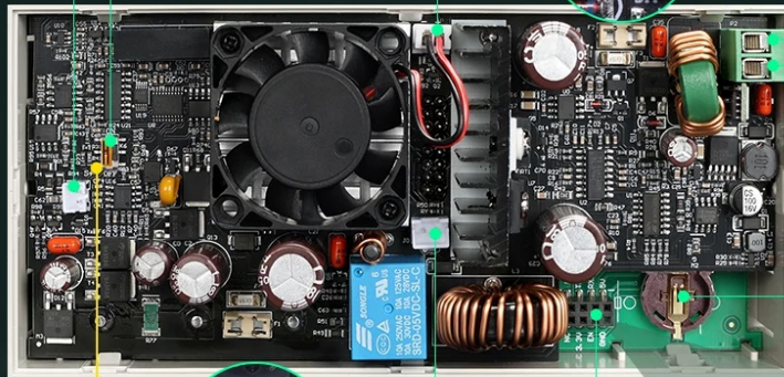
Clock Battery Slot (Please prepare CR1220 battery yourself)
