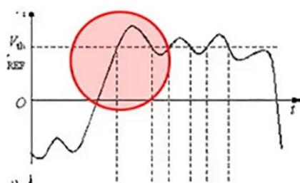
Take the high and low peaks within a cycle to calculate the average value, and the measurement results are calculated by the software average. Except for sine waves, other waveforms have significant errors.
