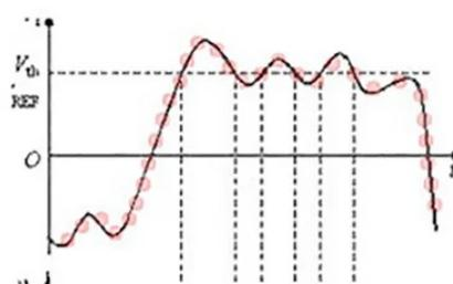
Hardware measures any waveform, and the measurement result is the true effective value, which can accurately measure all current waveforms
